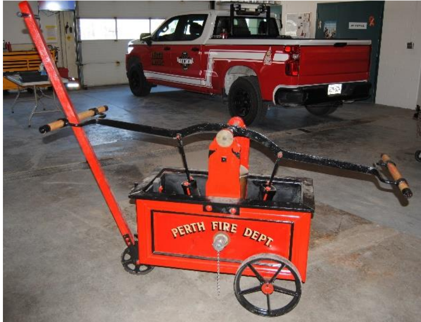
1842 'Murray' Fire Engine. The 'brakes' or push-bars on the pump handles are much shortened versions of the originals.
